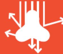
A trilobal fibre allows only a small proportion of light to pass through
