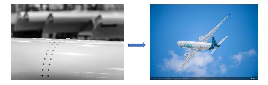
Manufacture of a complete slat with anticontamination coating on the leading edge by SONACA (min 6 months flight tests)
